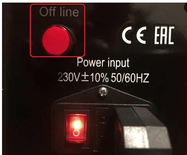
After the torch has been positioned, the „OFF line“ button must be pressed again, so that the light on the button does **NOT** on and the drives are switched on.
