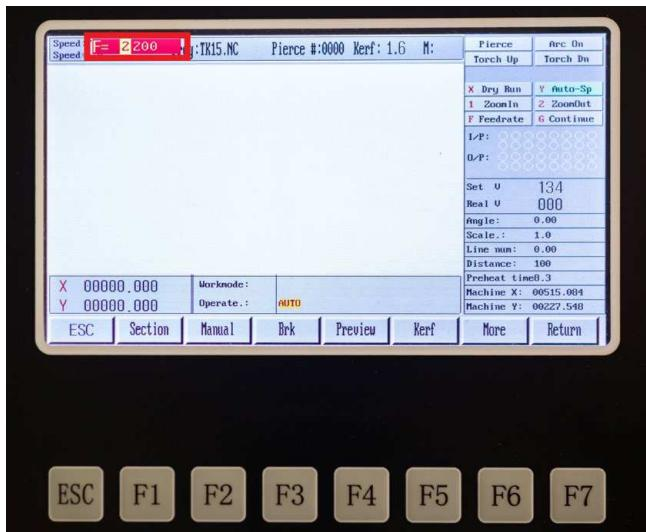
In the upper edge of the screen a field is displayed where the cutting speed is set with the numeric keypad. Then confirm with „Enter“.
