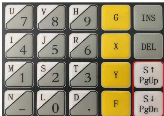
To make it easier to position the machine torch, the „S PgDn“ button can be used to move the torch down.
