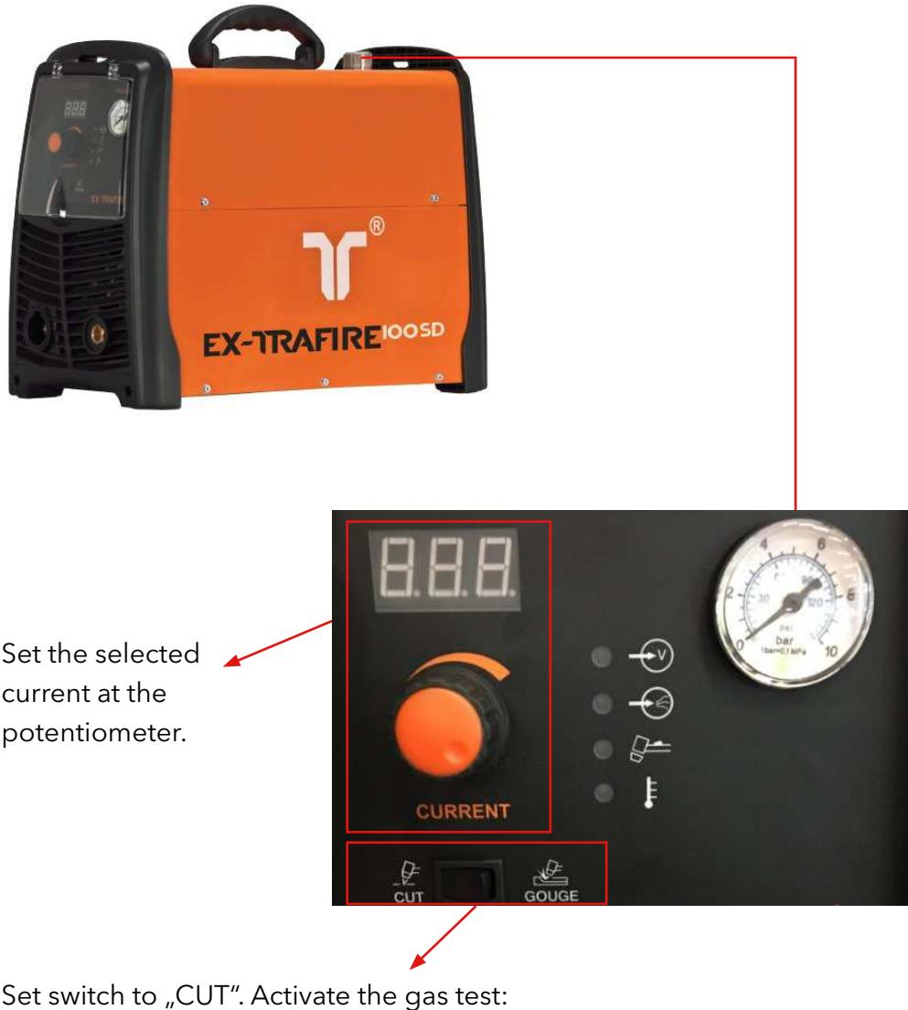
When changing the mode from "Cut to Gouge" and back, the system makes a gas test, where ideally the working pressure can be adjusted. During the gas test, set the cutting pressure (according to the FHT-EX® 105 RTX manual 5,2 Bar). Input pressure at the power supply is between 6- max. 10 bar.
