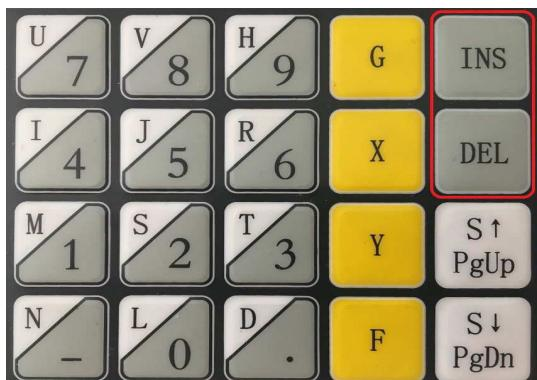
By pressing the „INS“ and „DEL“ button several times, the Arc voltage can be adjusted.
