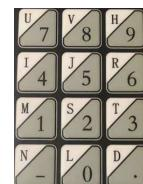
In the cutting data the value is given in mm. At the CNC control this value is entered in **time**. For example, at 4mm is 005 entered.
