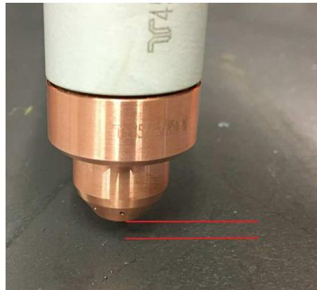
The ignition height is the distance between the shield cap and the material.
