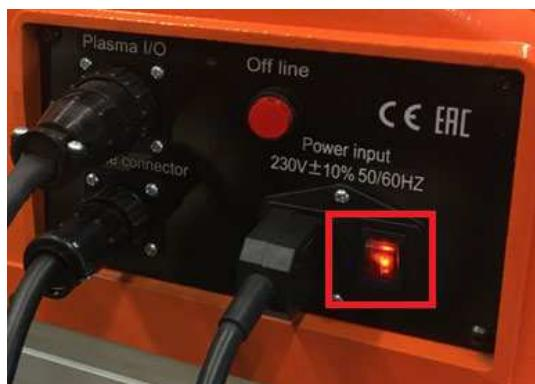
Switch on the CNC control at the on/off button.
