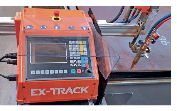
Display protection cover is made from 3mm polycarbonate and it is protection of display and keyboard of the EX-TRACK® CNC unit.
